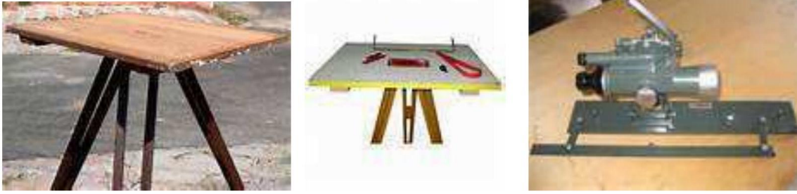
Figure 9: Plane table mounted on a tripod and Telescopic Alidade
