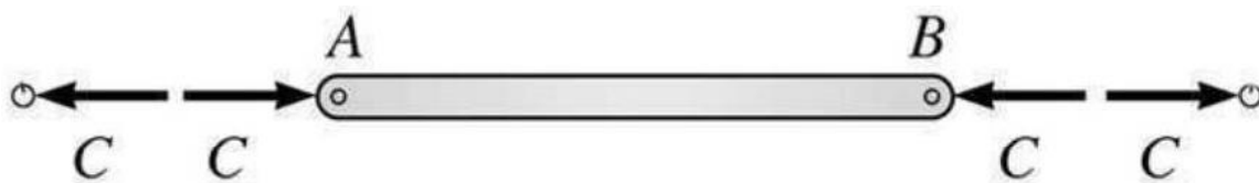
Figure 19 (c): Compression member of truss.
