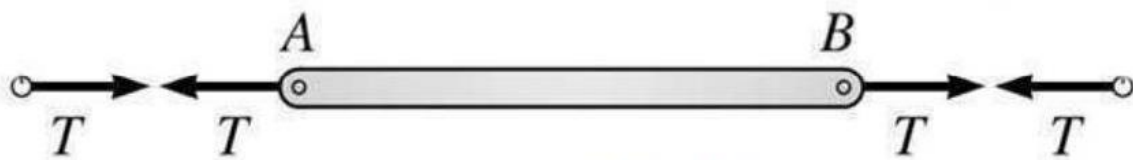
Figure 19 (b): Tension member of truss.
